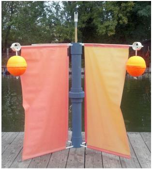
Standard hull with CODE floats and sails attached. Drifters can be field-rigged as either surface-following or deep-drogued.
