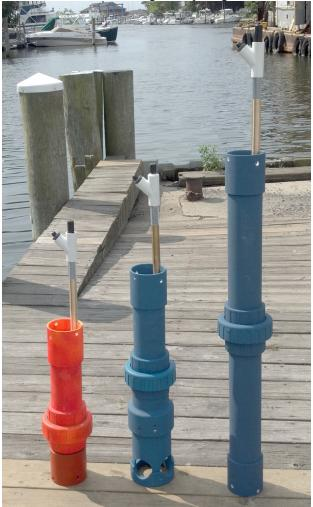
Left to right: mini hull, mini hull with conductivity/temperature sensor option, and standard hull.
