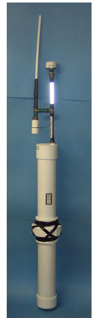
117 GPS mooring monitor with Argos telemetry
