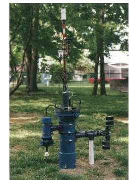
104 drifter with 24 sensor channels
